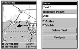
Trail selected with map cursor (left). The box at the bottom of the screen shows distance and bearing from current position to the selected point on the trail. The Edit Trail menu (right).
